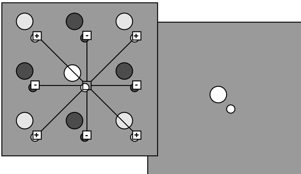
FIG. 1.—The logical filtering operation. An eight-point filter is passed over the image (left), whose output (right) is zero if the deviations from the mean background are not all in the same direction as that expected for a source aliased to the eight points in the co-add. Otherwise, the output is the pixel value at zero lag. This filter suppresses source aliases.
